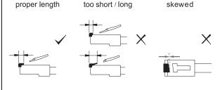
always check for proper fixing of the latch or it can cause jam in the jack!
